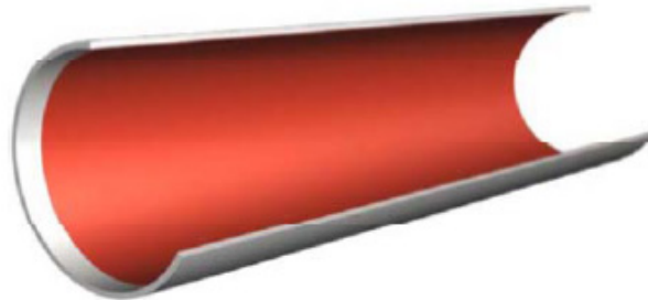
Figure 5.1 Internal pipeline coating will be an antifriction, epoxy-based coating.
