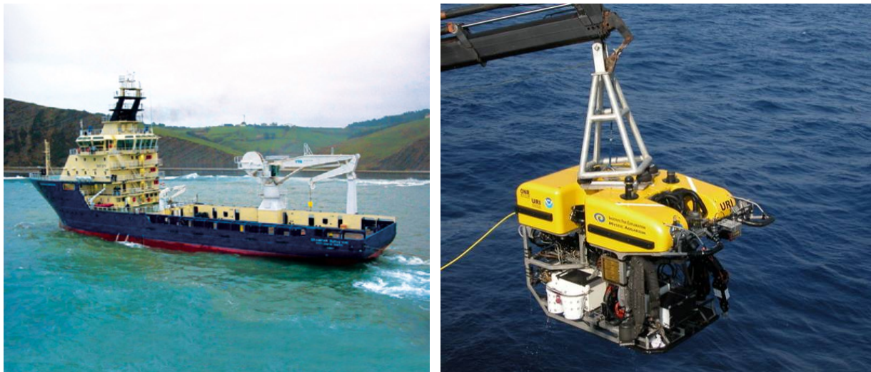
Figure 8.2 Typical survey vessel, the Saipem Grampian Surveyor (left) and ROV ready for launch (right). Photos by Saipem S.p.A.
